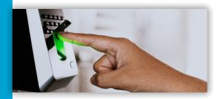
In built fingerprint scanner which enables the system to register personnel and identify them. Storage: Up to 3000 unique fingerprint storage per device.
